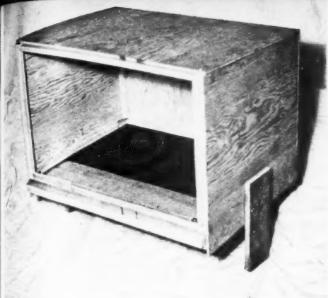
Front panel and motor mounting shelf consist of \frac{3}{4} in. plywood. Use \frac{1}{4} in. plywood for rest of housing and \frac{3}{4} in. wood strips for stiffening braces.
